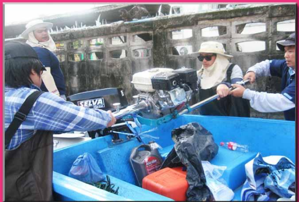
Teacher and students from Bangkok Bible Seminary are helping to install a long tail engine in a 5.3 M boat .
